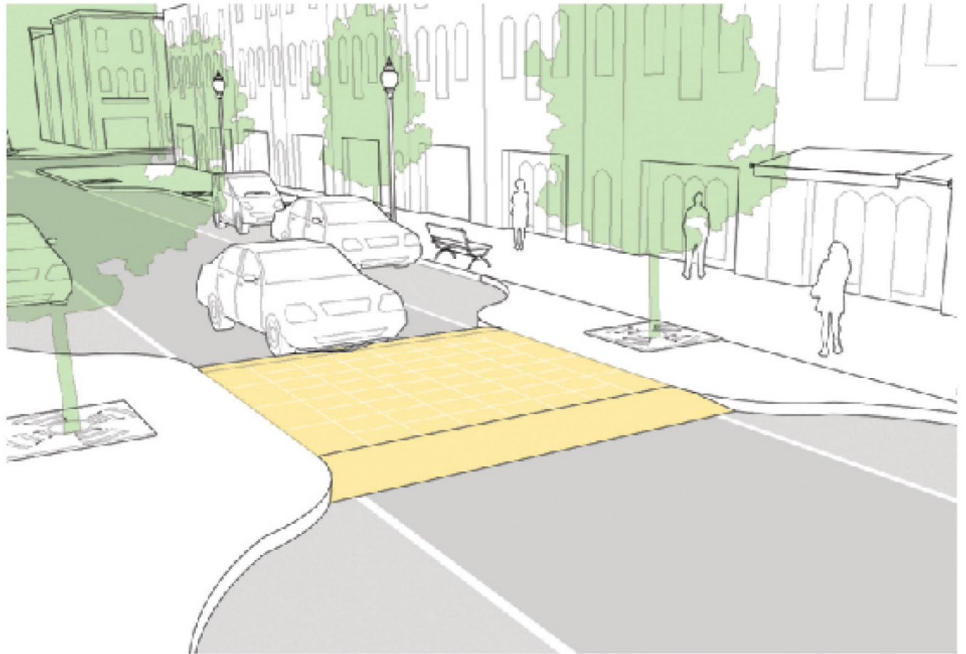
Proposed raised speed table example
